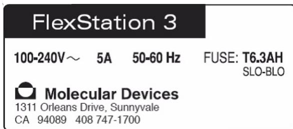
**Figure 1-2:** FlexStation 3 Instrument Label
