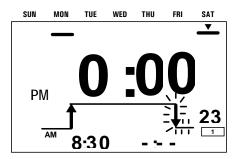
5. Using the h and m KEYS, set the time to 0:00 pm. Press the WRITE KEY to enter this setting into memory. The timer will display the complete operation for approximately one second, then the display will return to the initial PROG1 SET MODE DISPLAY, with the number of programmable operation steps remaining displayed in the lower right hand corner.
