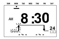
3. Press the **WRITE KEY** to enter this operation in memory. The timer will display the next operation to be programmed.
