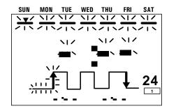
3. Using the **SHIFT** and **SET KEYS**, select the day of the week that the cycle operation is to start. In this example, the cycle is to be performed on Monday. Using the **h** and **m KEYS**, set the time the cycle operation will begin on Monday to 8:30 am. Press the **WRITE KEY** to enter this setting into memory.
