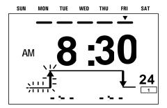
4. Press the **WRITE KEY** to enter this setting into memory. If the day, hour, and/or minute have not been set, the specified time and day will not be entered into memory when the **WRITE KEY** is pressed. Once the **WRITE KEY** is pressed, the timer will display the next available setting in **PROG1**. In this case, the timer will display the time the operation will stop.
