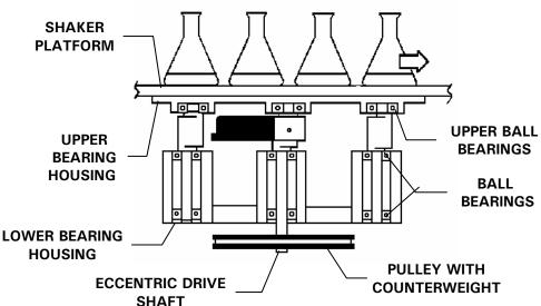
Figure 17: Bearing Housing Replacement
