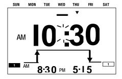
3. Open the lower drawer of the timer and press the **CHECK KEY**. Each time this key is pressed, the operation schedule is displayed in the sequence the operations are to be executed. The **ON** and **OFF** times for **PROG1** are displayed, starting with the earliest **ON** time. Then the times set for **PROG2** are displayed. After all the set times of both programs have been displayed, the timer returns to the **RUN** display.
