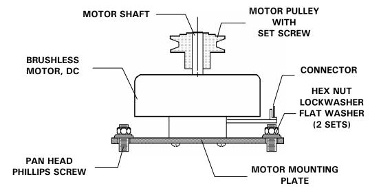
Figure 16: Motor Replacement
