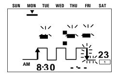
4. Using the **SHIFT**, **SET**, **h** and **m KEYS**, set the day and time the timer will stop the cycle operation. In this example, the timer will cease to cycle on Monday at 5:15 pm. Press the **WRITE KEY** to enter these settings into memory. The timer will then prompt you to input the cycle-on time.
