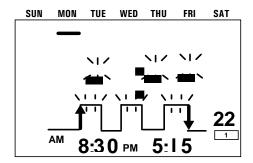
5. Using the h and m KEYS, set the span of time that the switch will be on to 0:02 (2 minutes). Please note that the cycle-on or cycle-off time cannot be set to 0:00. Press the WRITE KEY to enter this value into memory. The timer will then prompt for the cycle-off time.
