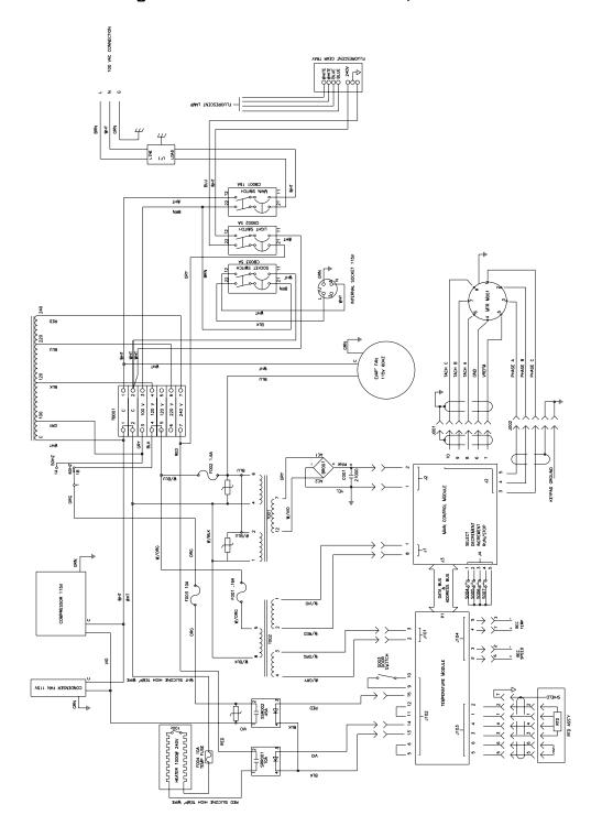
Figure 25: 100V Power Schematic, overview
