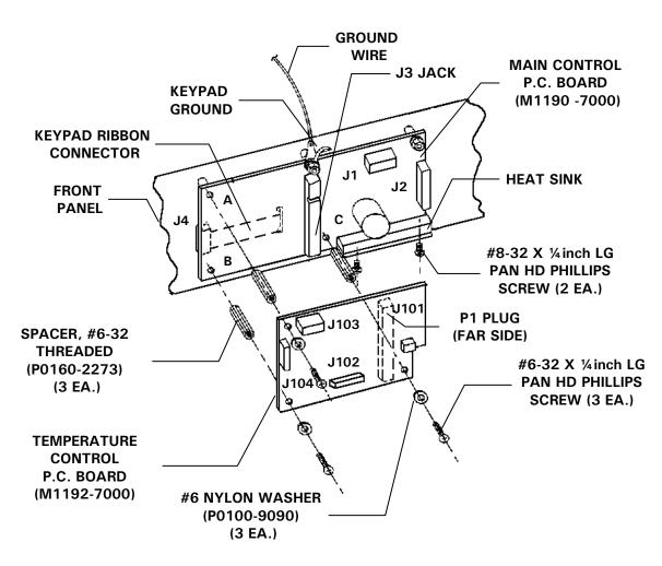
Figure 20: Temperature Board Replacement
