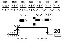
2. Open the lower drawer of the timer, and press the **CLR KEY**. The display will revert to the initial **PROG1 SET MODE DISPLAY**, and the number of steps remaining will be increased by the number of steps cleared in Program 1.
