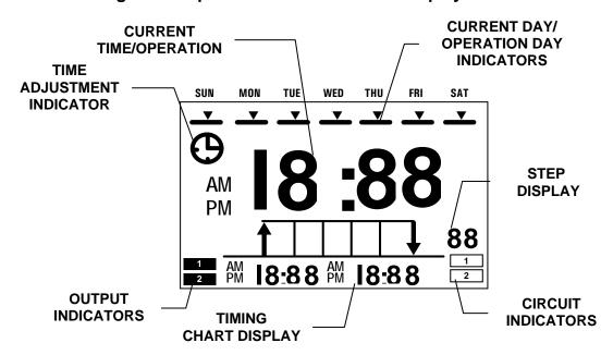
Figure 6: Optional Electronic Timer Display Detail
