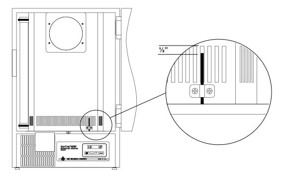
Figure 19: Temperature Sensor Adjustment
