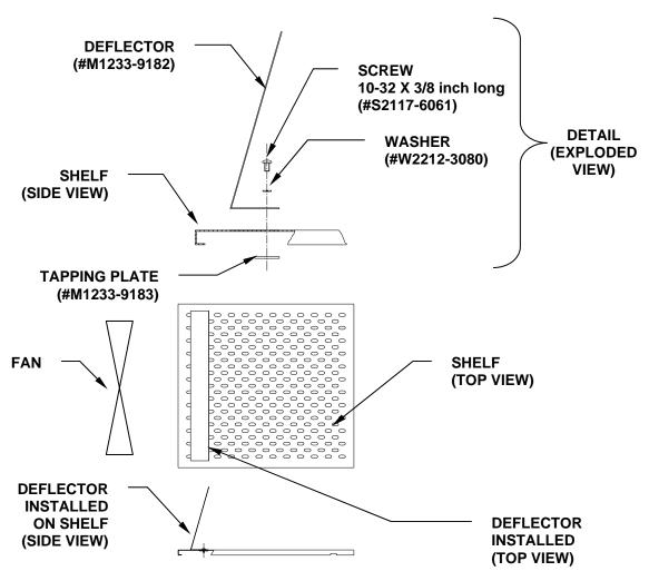
Figure 12: Air Deflector Installation
