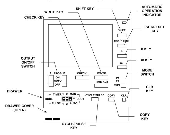
Figure 5: Electronic Timer (Optional) Detail
