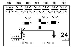
2. Open the lower drawer of the timer by pulling the cover down, and press the **CYCLE KEY**. The timer will enter the **CYCLE PROGRAM MODE**.
