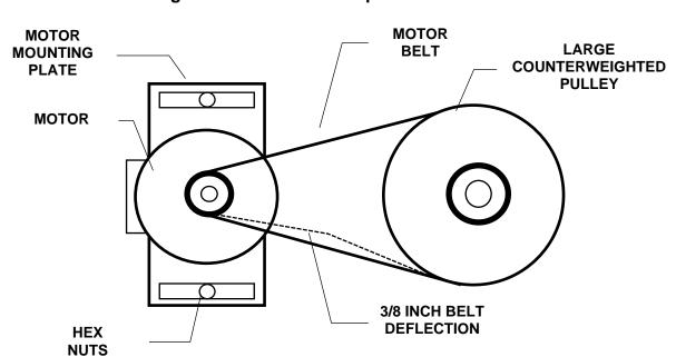
Figure 15: Motor Belt Replacement
