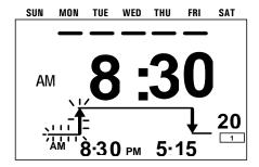
3. Continue to press the **WRITE KEY** to view the programmed (set) times. After all the operations have been displayed, the initial **PROG1** display will appear in the display.
